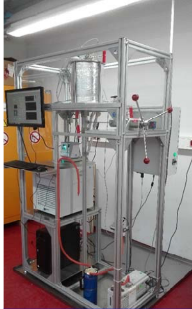
Density measurements up to 4000 bar and temperatures up to 200 °C
