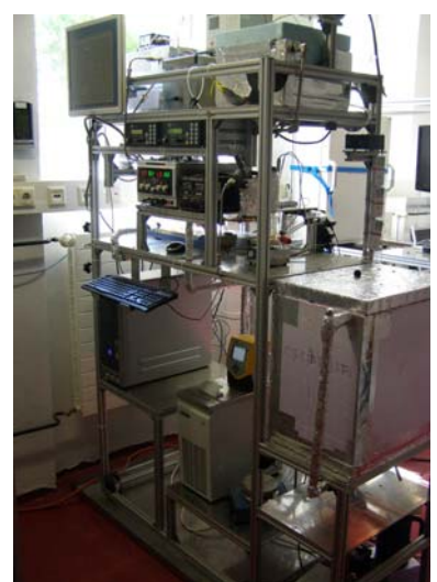
Vapor pressure measurements at small temperatures
