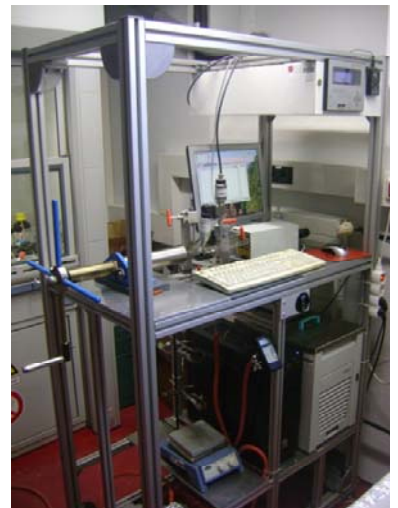
Density measurements up to 1400 bar and temperatures up to 200 °C
